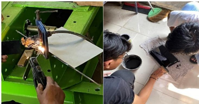
Figure 3. Small Barricade Welding and Painting Process
